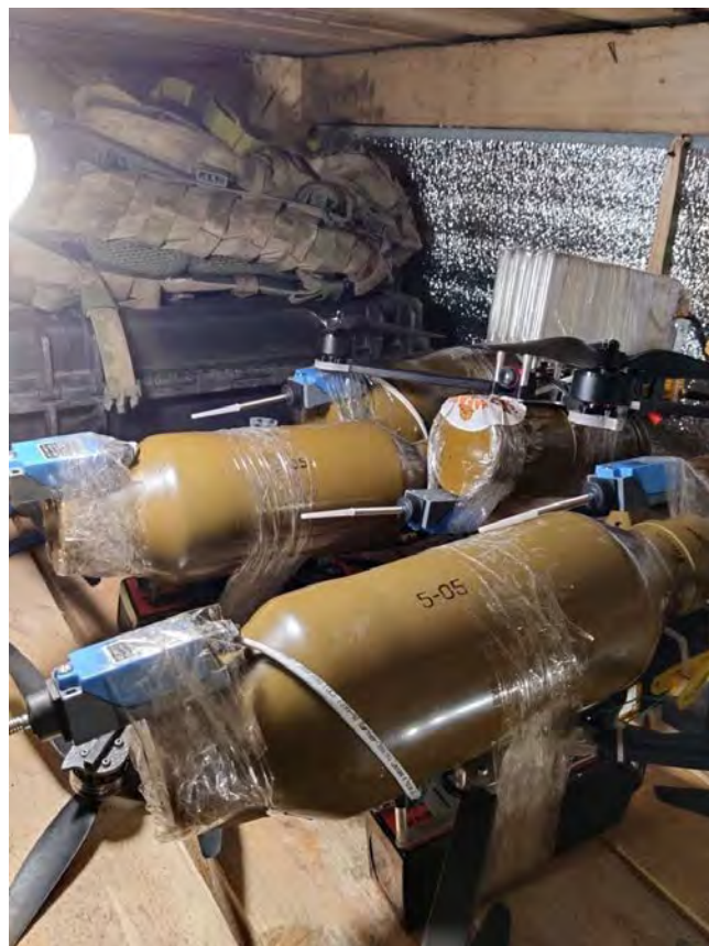
Figure 3 – Russian FPV drones fitted with improvised munitions based on a modified TBG-7V thermobaric rocket warhead / cheap COTS microswitch used in the device (Source: @VictoryDrones & Aliexpress.com)
