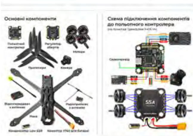
Figure 2 – FPV drone main components (Source: @VictoryDrones)
