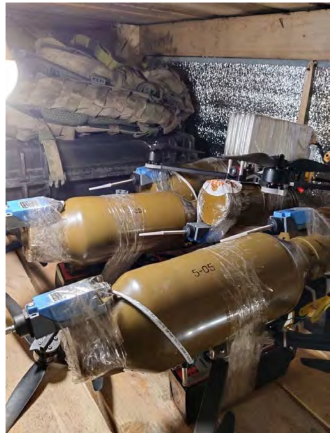
Figure 3 – Russian FPV drones fitted with improvised munitions based on a modified TBG-7V thermobaric rocket warhead / cheap COTS microswitch used in the device (Source: @VictoryDrones & Aliexpress.com)
