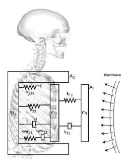
Figure 4. Spring-Mass-Dashpot compact model of thoracic biomechanics and impact injury (based on Lobdell et al. 1973; Viano 1978; Viano & Lau 1988; Stuhmiller et al. 1996).
