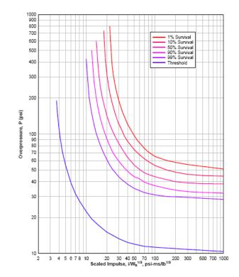
Figure 3. Survival Curves for Lung Damge, Wh = Weight of human being (lbs) UFC 3-340-02
