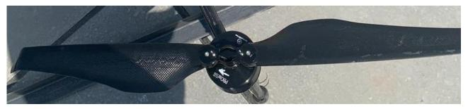
The motor minimum specifications (for 100KV version) indicate a maximum payload of 10 Kg at least for a quadcopter design.
