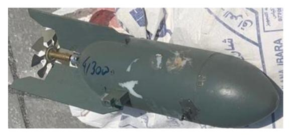
The three-fin design is quite strange, and not identifiable as any already known conventional aerial bomb. No fragmentation enhancement is reported (the low weight of the munition is not pointing at any fragmentation effect too).
